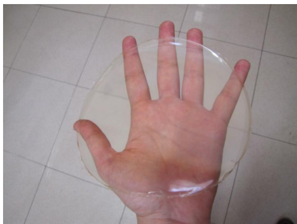
Fig. 1. Appearance of soluble soybean polysaccharide based film (30% w/w glycerol was used in its formulation).
